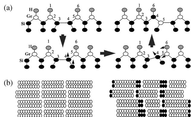
FIG. 3. Atomistic models of the proposed place exchange mechanism and structure. (a) Dimer-vacancy diffusion-assisted Si-Ge place exchange reaction. When a vacancy moves one step, two Si atoms are brought to the surface. (b) A top view of the  $(2 \times N)$  reconstructed surface before and after Si segregates to the surface at the vacancy lines. The dimer rows run horizontally; Si, occupying surface sites in the vicinity of the vacancy lines, produces a striped phase (vertical dark bands).
